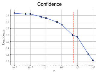
Figure: Effect of the temperature for a Resnet20 trained on CIFAR-10. No cooling \eta_N = 1 is indicated by a red line.
